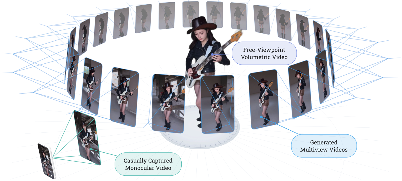
Fig. 1. Given a casually captured monocular video, typically with mild camera motion and unknown camera intrinsics and poses, 4DAnyone generates multiview-consistent human videos, enabling 4DGS reconstruction rendered from free viewpoints. See the project page and Fig. 7 for more results.
